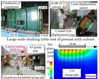
In-situ lateral loading test on 63 group pile and it's FEM
