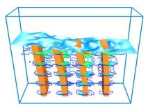
Fig. 3 : Deformation of elastic plates due to sloshing fluids
