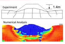
Fig. 1. Deformation of an embankment resting on liquefiable ground (Centrifuge experiment and numerical analysis)
