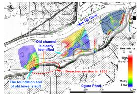
Fig. 2 : Contours of resistivity superimposed on to an old topographical map, published in 1921 by Kyoto City
