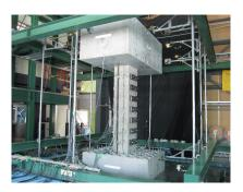
(d) Dynamic experiments of high-capacity structure piers.
