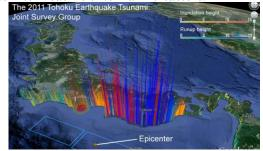
Survey data of tsunami run-up around Japan coast by the 2011 Tohoku Earthquake tsunamis
