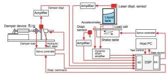
Hybrid simulation of fluid-structure-device system
