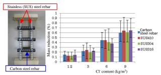
Galvanic coupling between carbon steel and stainless steel in concrete containing high amount of chloride ion
