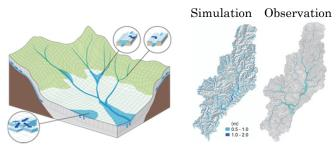
Rainfall-Runoff-Inundation Model (left) and its application (right)
