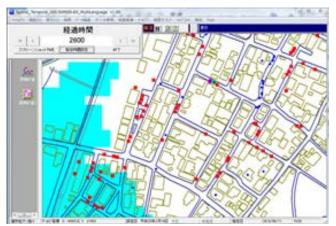
Tsunami Evacuation Evaluation System based on Multi-Agent Simulation
