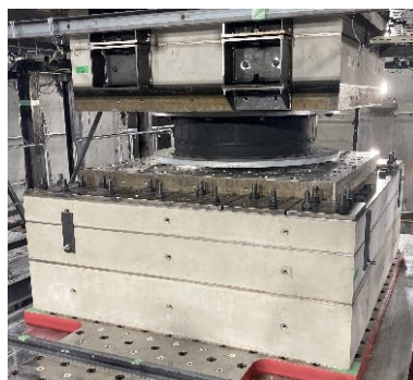
Loading test of full-scale seismic isolation bearing (φ1200mm)
