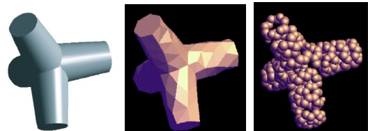
Fig. 3 : T-type solid model (Left: CAD, Center: tetrahedron elements, Right: CDS)
