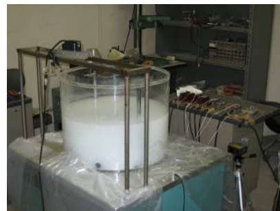
(a) New device preventing a liquid sloshing behavior.
