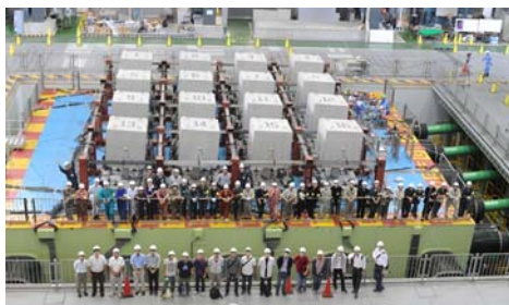
Simultaneous Excitation of 16 RC Piers at E-Defense
