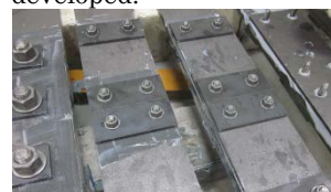
Improvement of long-term behavior by setting bolt
