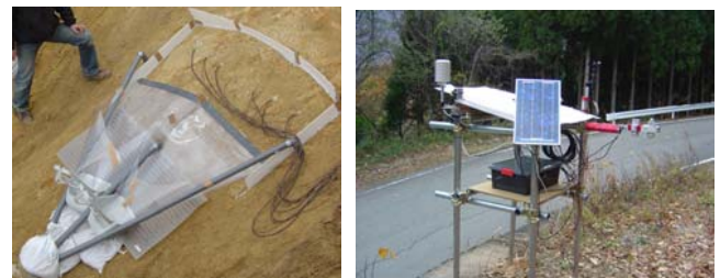
Fig. 2 : Field observation of both sediment production rate and meteorological conditions
