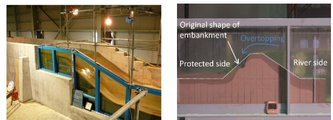
Experimental flumes for the river dyke breach (left) and landslide dam (right) in Ujigawa Open Laboratory
