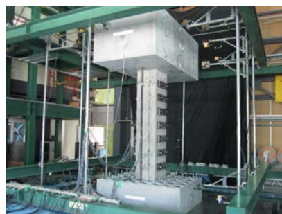
(b) Dynamic experiments of high-capacity structure piers.
