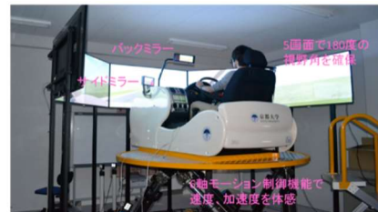
Driving simulator equipped with 6-axis motion
