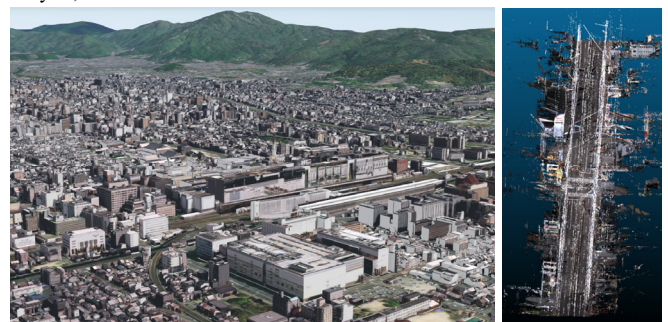
Example visualizations: 3D city model of Kyoto City using the Ministry of Land, Infrastructure, Transport and Tourism's 'PLATEAU' project (left), and road space representation using point cloud data provided by Shizuoka Prefecture's 'VIRTUAL SHIZUOKA' (right).
