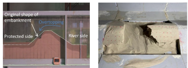
Experiments on the river dyke breach (left: one-dimensional flume in the cross-sectional direction, right: two-dimensional flood basin with river flow)
