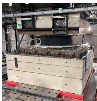
Loading test of full-scale seismic isolation bearing (φ1200mm)
