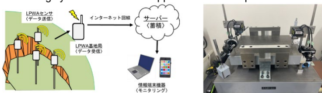
Overview of slope monitoring using LPWA with lab test
