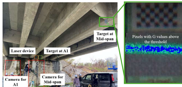
On-site experiment on Laser and Video based measurement
