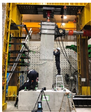
Loading test of a large RC column specimen
