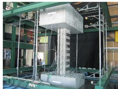
(d) Dynamic experiments of high-capacity structure piers.
