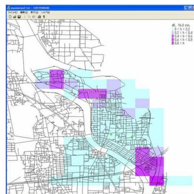
Fig. 2 : Flood evacuation simulation model based on digital modeling of street network.
