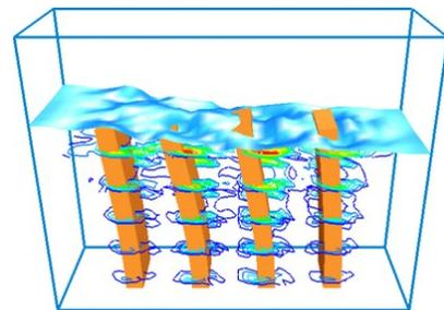
Fig. 3 : Deformation of elastic plates due to sloshing fluids
