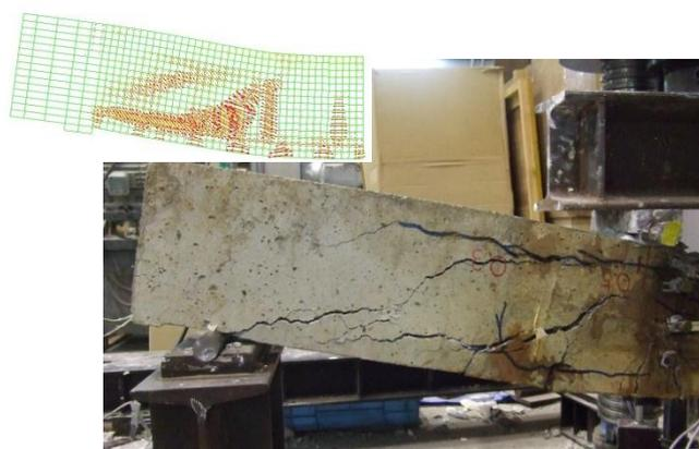
Fig.2 Flexural loading test and FE analysis of RC beam with the corroded reinforcements
