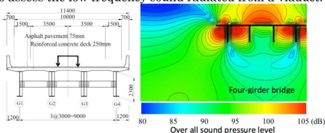
Fig. 2: Simulated sound propagation radiated from four-girder bridges.
