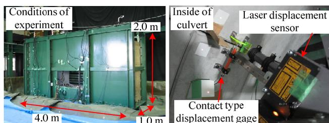
Large scale shaking table test of precast arch culvert
