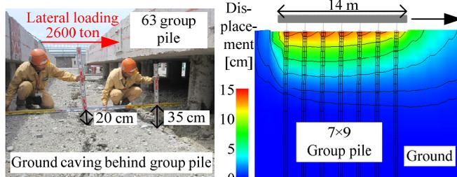
In-situ lateral loading test on 63 group pile and it's FEM
