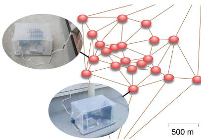
(b) Super-dense seismic array observation in Furukawa area.
