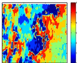
DMD analysis of velocity fields in bottom layer of a separation bubble.
