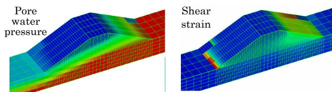
Simulations by the seepage- deformation coupled
