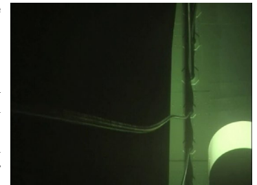
Rain-wind induced vibration of a stay-cable
