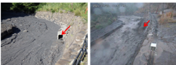
Fig. 2: Observation equipment in debris flow-prone stream to observe the fine sediment content rate in debris flow.
