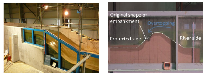
Experimental flumes for the river dyke breach (left) and landslide dam (right) in Ujigawa Open Laboratory
