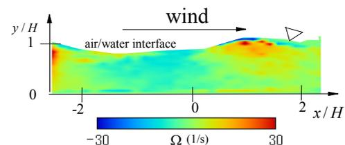
Fig. 3 : Coherent vortices in wind-induced open-channel flows
