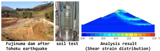
Fig. 1 : Investigation of failure mechanism of Fujinuma dam
