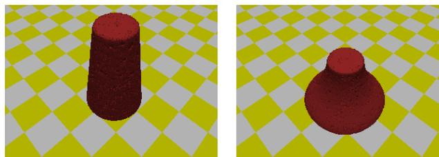
Fig.: Simulation of concrete slump test
