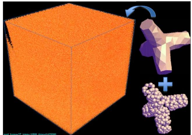
Fig. 4 : 1 million blocks in 3D cavity flows taking account of the collisions of blocks and fluid-structure interactions (4,096 parallel computations with CRAY XE6 in Kyoto University); right figures show each block and CDS included in a block.
