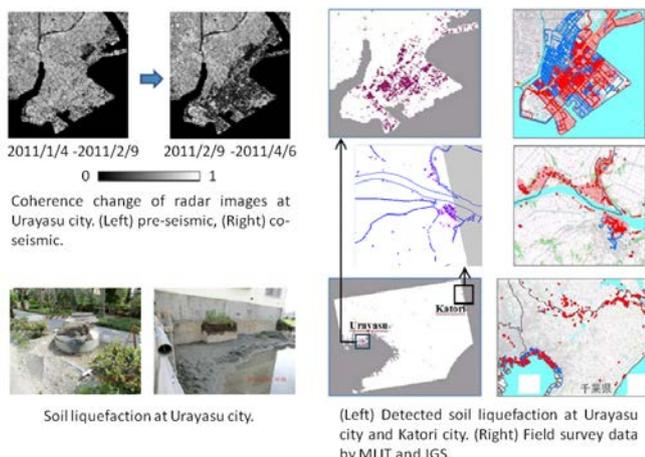
Detection of liquefaction areas in Kanto region caused by the 2011 East Japan Earthquake. Liquefaction areas were detected using ALOS-PALSAR radar interferometry.
