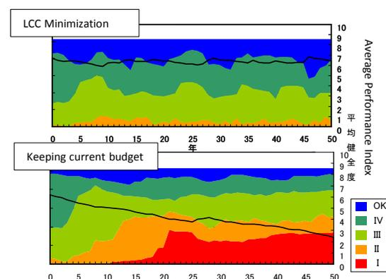
Fig 2. Life Cycle Cost Minimization using Bridge Management System
