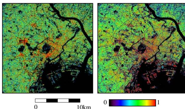
(Left) urban density estimated by using SAR data and (right) building-to-land ratio from GIS data in Tokyo area
