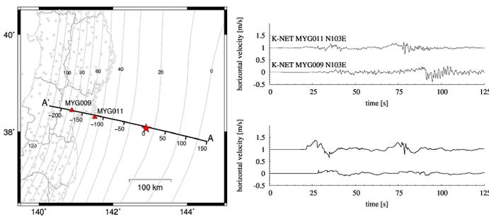
(a) Rupture simulation for the 2011 great Tohoku earthquake.
