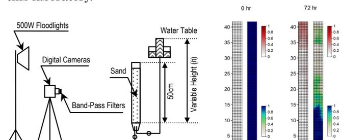
Fig. 2: Experimental setup for testing the migration of a contaminant in a one-dimensional column
