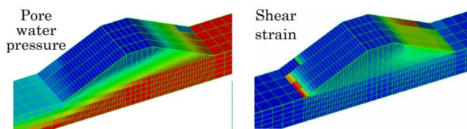
Simulations by the seepage- deformation coupled
