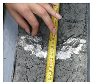
Gas hydrate bearing sediments from Lake Baikal
