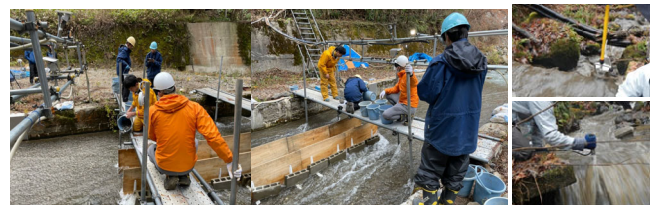
Fig. 3 : Field experiment with hydrophone and other equipment to observe bed load in Hodaka Sedimentation Observatory
